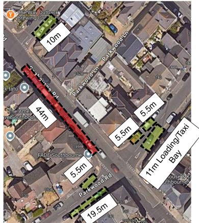
Remove existing 44m parking section. Replace with 'No Waiting At Any Time' Parking Restriction.
